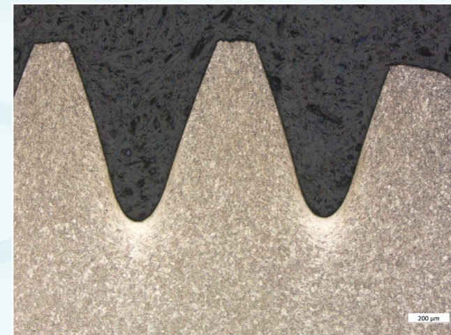
Stainless Steel fastener, external electrolytic etching with 10% aqueous oxalic acid, BF, 50x
