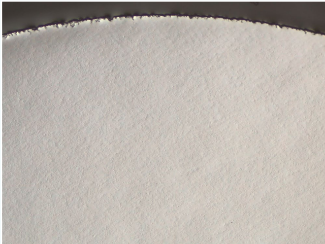
Pure Titanium, Grade 4, DIC, 100x
