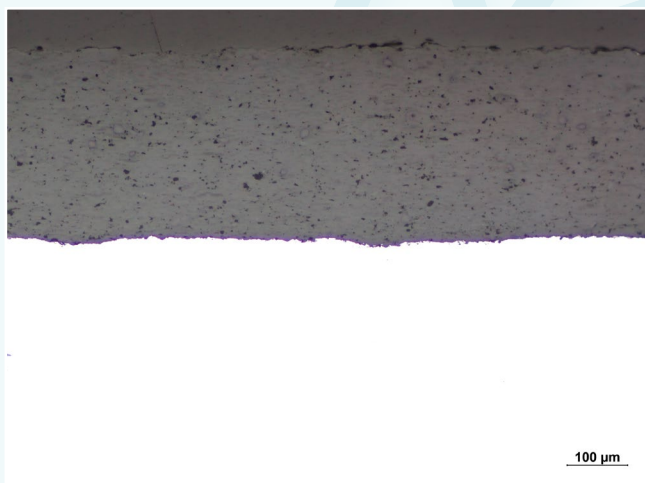
Al 2 O 3 coating on a steel substrate, BF, 100x
