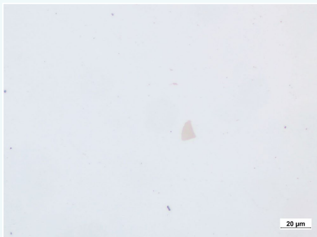
Tool Steel X40CrMoV51+QT, 410-470 HV, cross section BF, 500x
