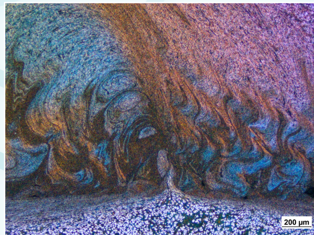
Aluminium friction stir weld, etched according to Barker, POL + Lambda Compensator, 50x
