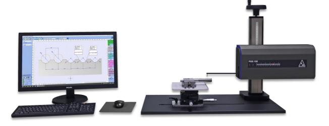
The PGS100 profilometer allows to acquire 2D profiles in an extremely simple and intuitive way, thanks also to its measuring range of 130 mm in length (X) and 50 mm in height (Z).
