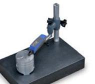
Granit basement 400x250 mm and positioning column, maximum measuring height respect to the plane: h=150 mm.
