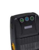
Portable thermal printer with Bluetooth connection to print parameters and charts of the measure.
