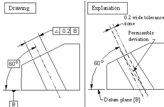
Define plane 1 on datum face [B], and cylinder 1 in the angled hole as per the drawing above. Select Measure from the tool bar
