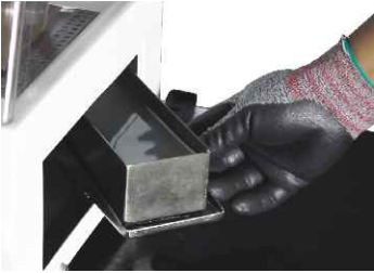
Easy movable Built-in Re-Circulation Coolant Tray
