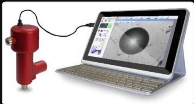
CAMÉRA PORTABLE EASYBRINELL POUR LA LÉCTURE ET LA MESURE BRINELL
