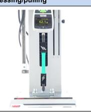
This unit graphs the process and enables you to visually check the force transition until the sample is broken. Also, it helps you to easily find the force/displacement value and peak value when the sample is broken, and leave a comment.
